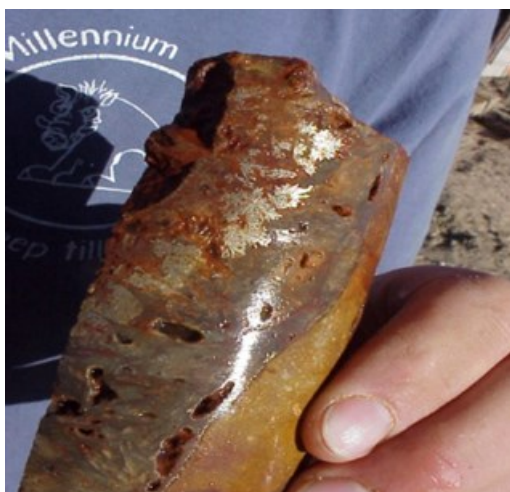
Drill core showing free gold
