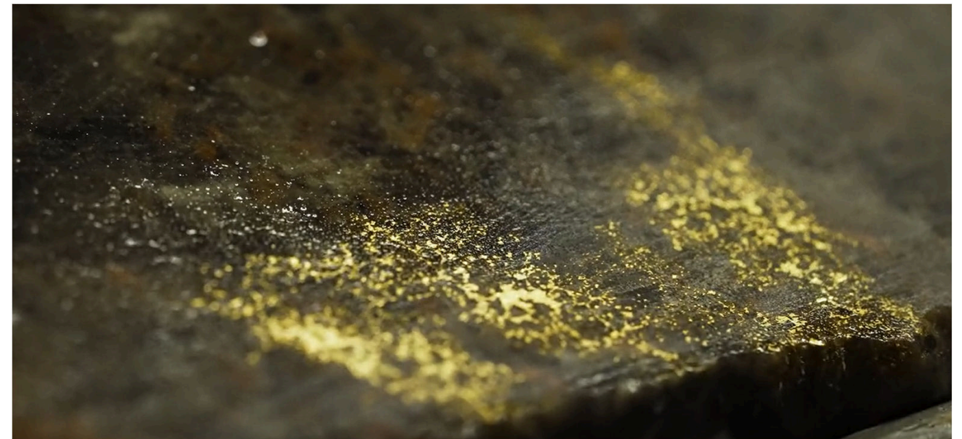
Visible Gold (VG) in drill hole DO-05-04. Part of sample that returned 2,888 g/t Au over 0.5m at Douay
