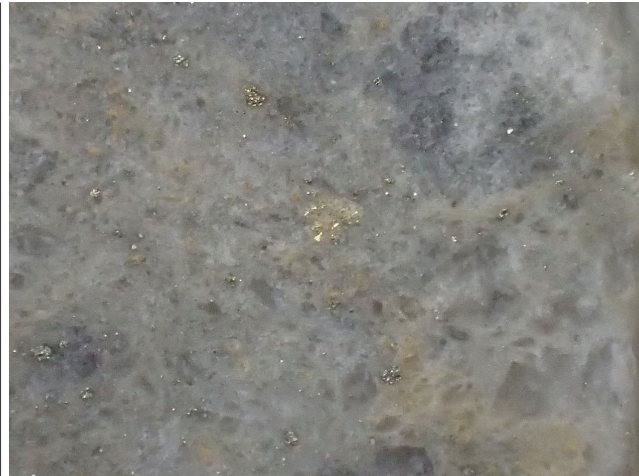
Cluster of high reflectance visible gold grains at 307.6m in DO-21-310, part of sample interval grading over 8g/t Au. Note abundant silica content with crystal fragments that contrasts with the apparent basaltic composition of the host rock.
