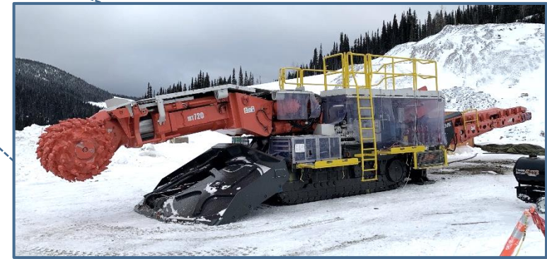
ROADHEADER AT SITE
