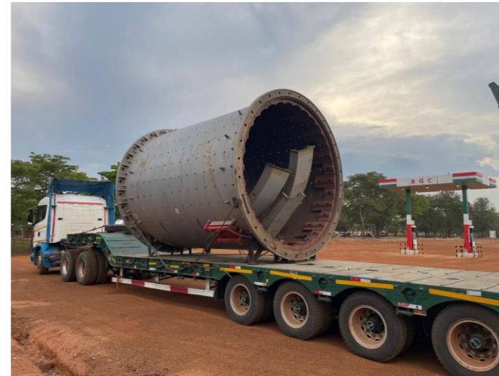
Figure 1. Arrival of the new 1,000 tpd ball mill
