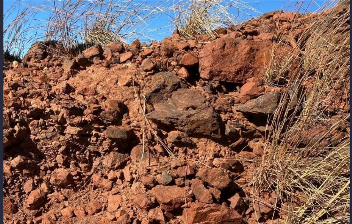
Trench 36: High-grade lump and fines iron ore DSO weathered zone, 2.2m at ~66% Fe*
